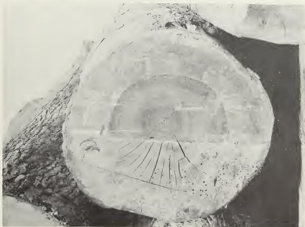
Figure 17. --Effect of end coating in preventing end checking in the right half of a sweetgum log.
